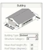
End Zone Calculation Min. Building Dimension (ft): 45 End Zone Distance (ft): 4.5
